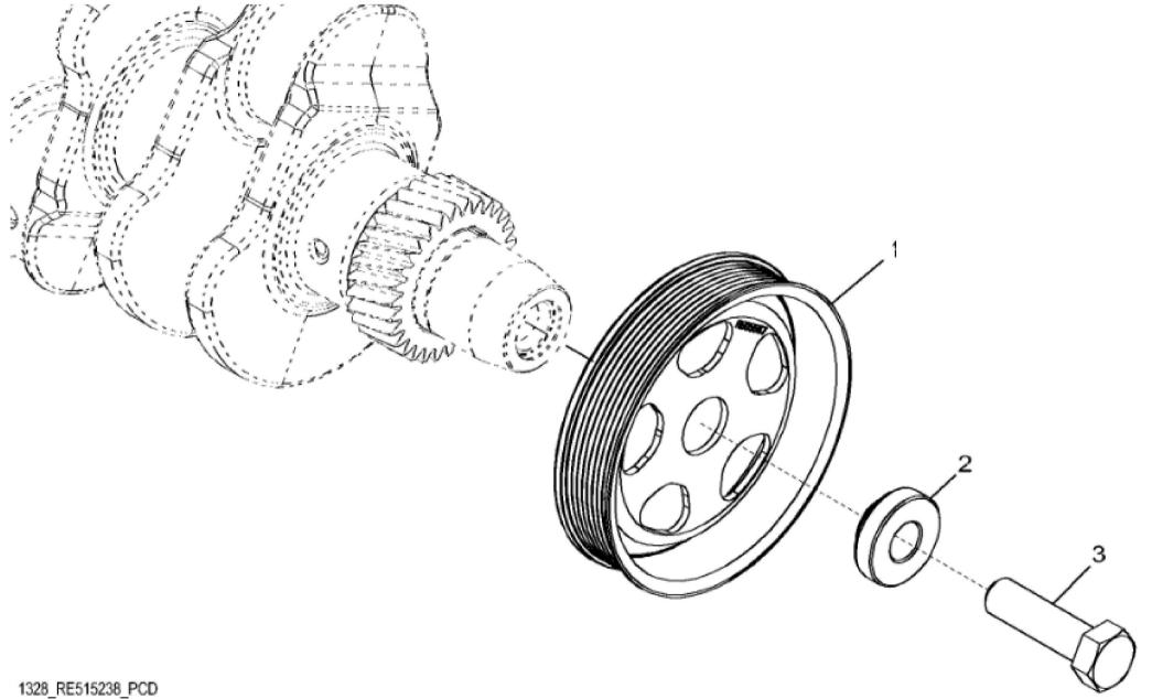
John Deere > Construction And Forestry >BACKHOE, LOADER >410L - BACKHOE, LOADER >410L Backhoe Loader (Engine 4045HT087, 4045TT096)(PIN: 1T0410LX\_\_C273920- )(PIN: 1T0410LX\_ \_D273920- ) >04A ENGINE 4045HT087-RE566133 >0400A ENGINE 4045HT087-RE566133 4045HT087 >ST628039 - 1328 CRANKSHAFT PULLEY
