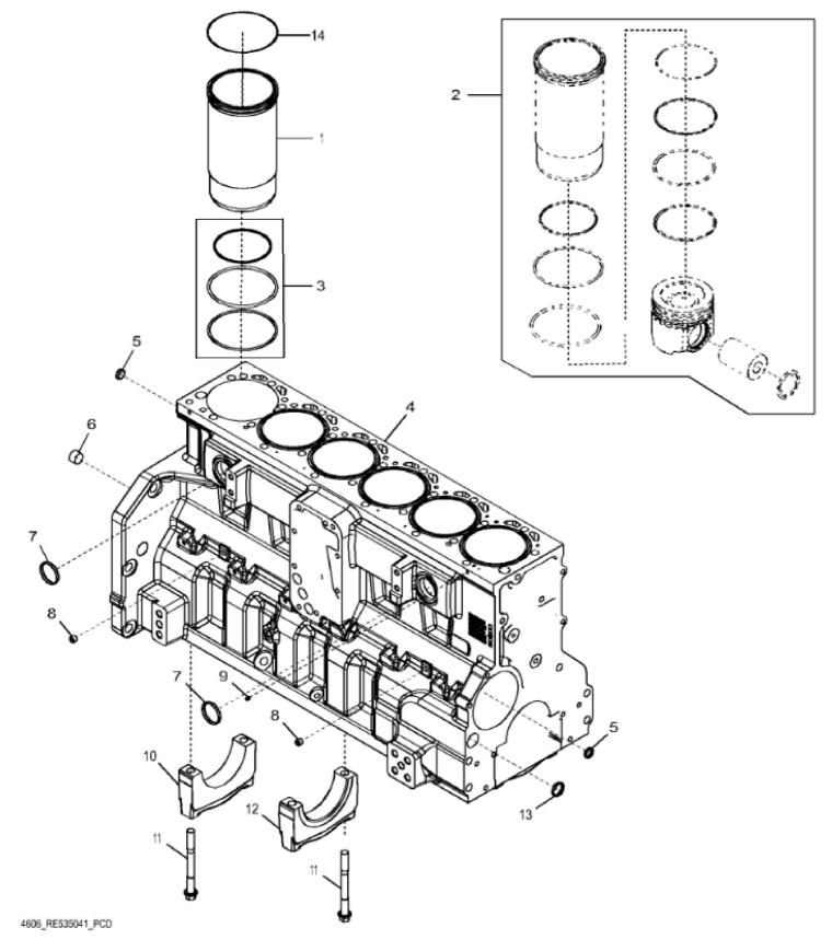
John Deere > Agriculture >TRACTOR >9460R - TRACTOR >9460R Tractor (S.N. 000101 - 001999)(Russian Edition) >20 ENGINE 6135RW201-RE541635 >ST132522 - 4606 CYLINDER BLOCK WITH LINERS
