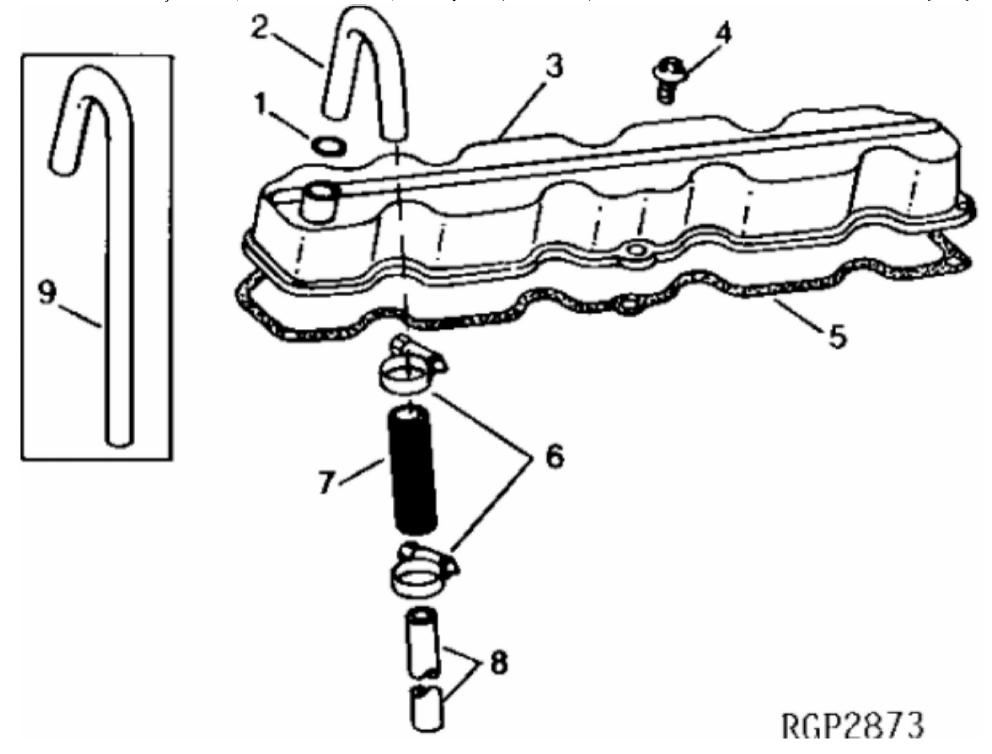
John Deere > Construction And Forestry >BACKHOE, LOADER >500A - BACKHOE, LOADER >JD500-A (123114-152141) Backhoe Loader >10 ENGINE >10-12 - ROCKER ARM COVER [01B13]
