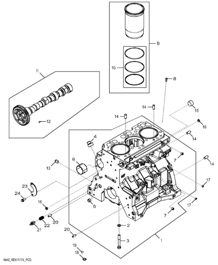
John Deere > Turf And Utility >TRACTOR >3029HPY62 - TRACTOR >5055E Tractor (Final Tier 4)(9X3 TSS Transmission and 12X12 PR Transmission)(North America Edition) >20 ENGINE 3029HPY61-RE571749 >ST799395 - 46AZ CYLINDER BLOCK
