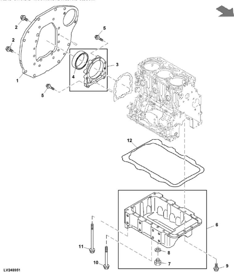
John Deere > Turf And Utility >TRACTOR, COMPACT UTILITY >3TNV84T - TRACTOR, COMPACT UTILITY >3038R Compact Utility Tractor >20 ENGINE >ST767242 - MOUNTING FLANGE AND OIL SUMP
