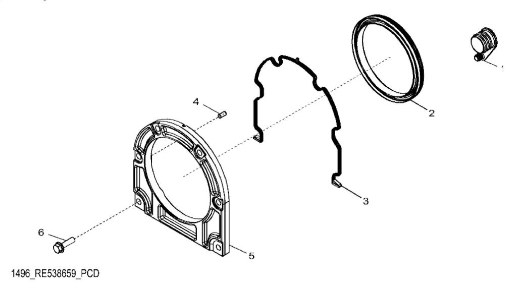
John Deere > Agriculture > TRACTOR > 9370R - TRACTOR > 9370R Tractor (S.N. 015000-) (Worldwide Edition) > 20 ENGINE 6090RW222-RE553208 > ST122156 - 1496 CRANKSHAFT OIL SEAL AND HOUSING
