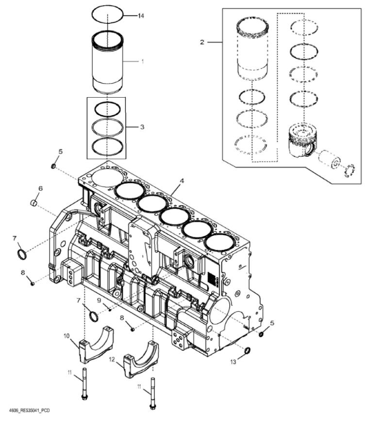
John Deere > Agriculture >TRACTOR >QSX15 - TRACTOR >9570R Tractor (S.N. 015000-)(Worldwide Edition) >20 ENGINE 6135RW203-RE553209 >ST132522 - 4606 CYLINDER BLOCK WITH LINERS
