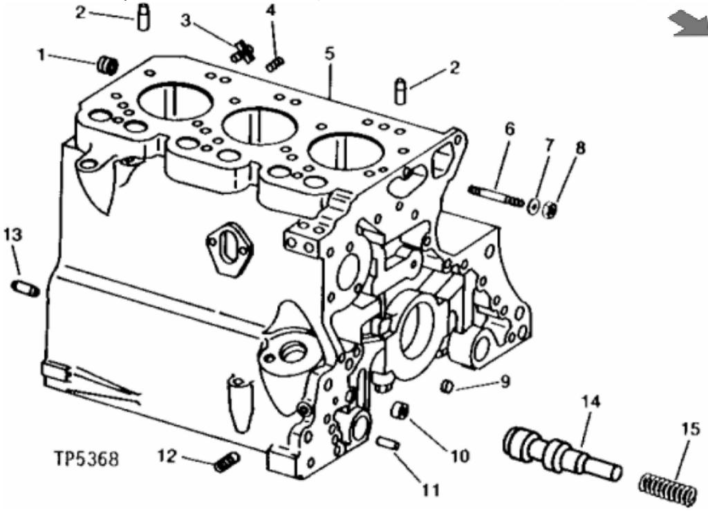
John Deere > Construction And Forestry >BACKHOE, LOADER >310 - BACKHOE, LOADER >JD310 Backhoe Loader >10 ENGINE >10-1A - CYLINDER BLOCK (SERIAL NO. -169357) [01A20]
