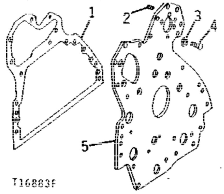
John Deere > Construction And Forestry >BACKHOE, LOADER >310 - BACKHOE, LOADER >JD310 Backhoe Loader >10 ENGINE >10-2 - ENGINE FRONT PLATE [01A24]
