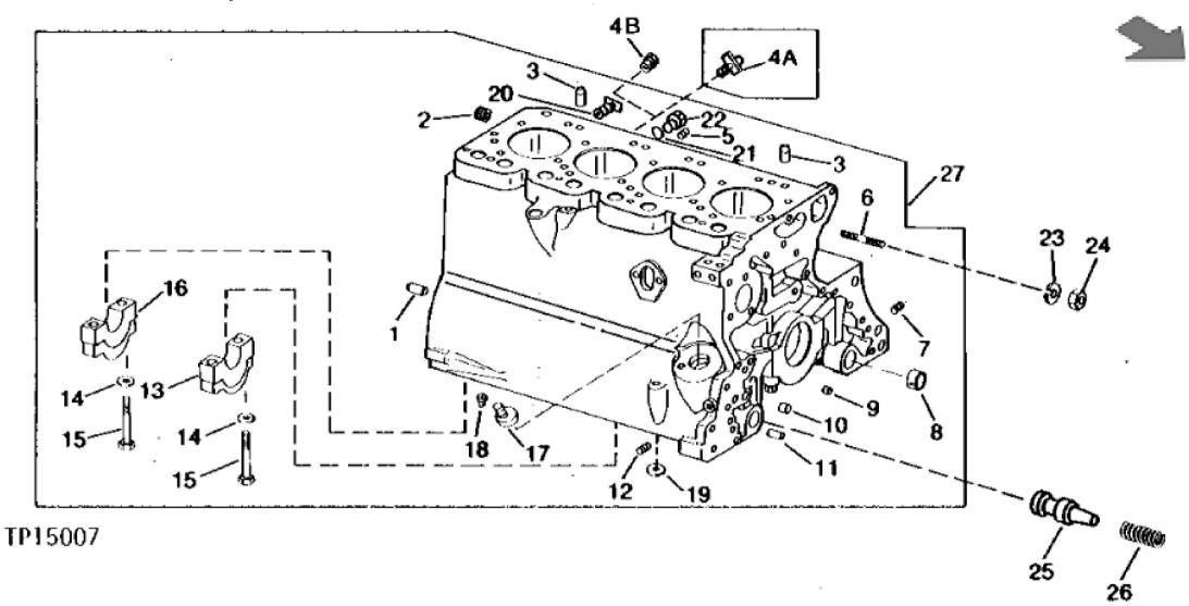
John Deere > Construction And Forestry >BACKHOE, LOADER >410 - BACKHOE, LOADER >410 Backhoe Loader >10 ENGINE >10-1C - CYLINDER BLOCK (SERIAL NO. 192001-) [01B05]
