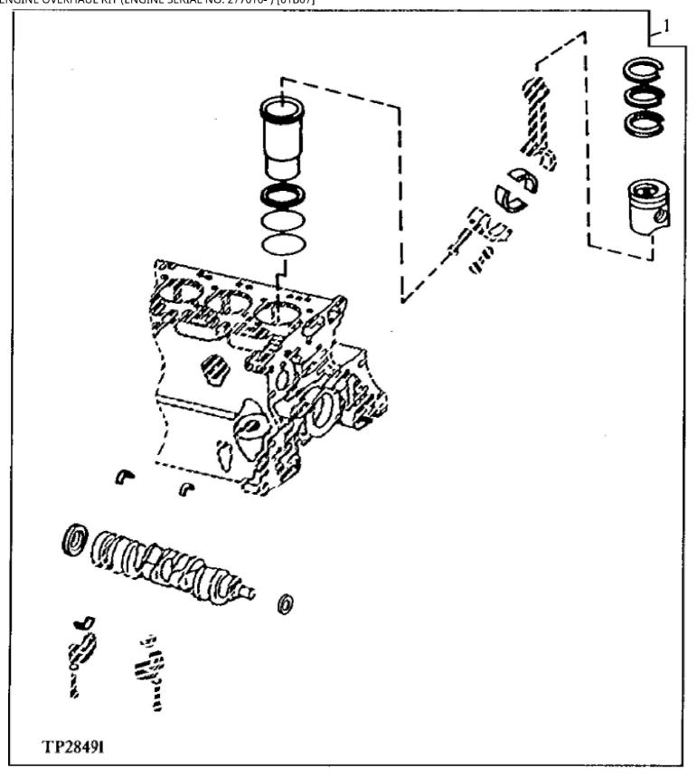
John Deere > Construction And Forestry >BACKHOE, LOADER >410 - BACKHOE, LOADER >410 Backhoe Loader >10 ENGINE >10-1E - BASIC ENGINE OVERHAUL KIT (ENGINE SERIAL NO. 277616-)
