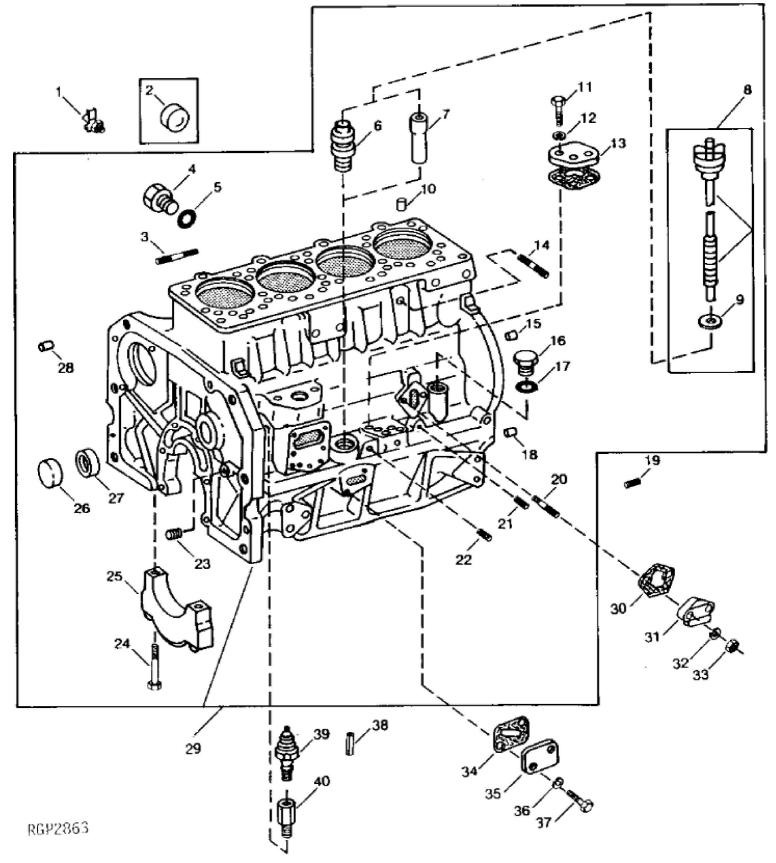
John Deere > Construction And Forestry >BACKHOE, LOADER >500C - BACKHOE, LOADER >500C Backhoe Loader >10 ENGINE >10-12 - CYLINDER/SHORT BLOCK, MAIN BEARING CAPS, DIPSTICK AND ENGINE OVERHAUL KIT - CONTINUED [01B14]
