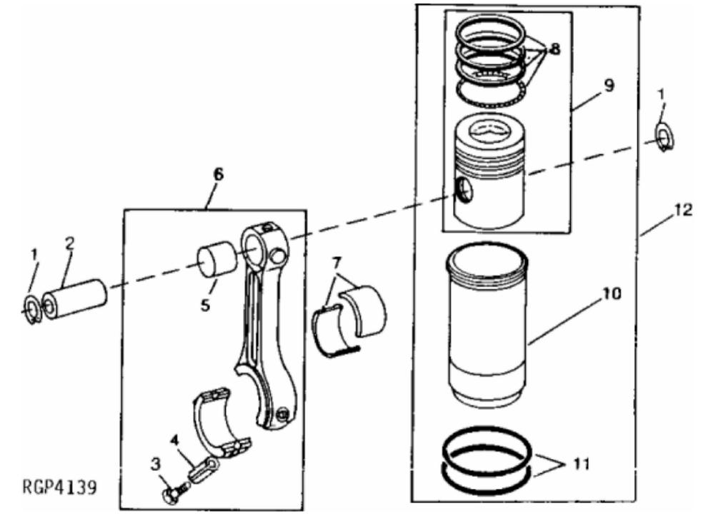
John Deere > Construction And Forestry >BACKHOE, LOADER >500C - BACKHOE, LOADER >500C Backhoe Loader >10 ENGINE >10-14 - PISTONS, RINGS, LINERS AND CONNECTING RODS (DIESEL) [01B16]
