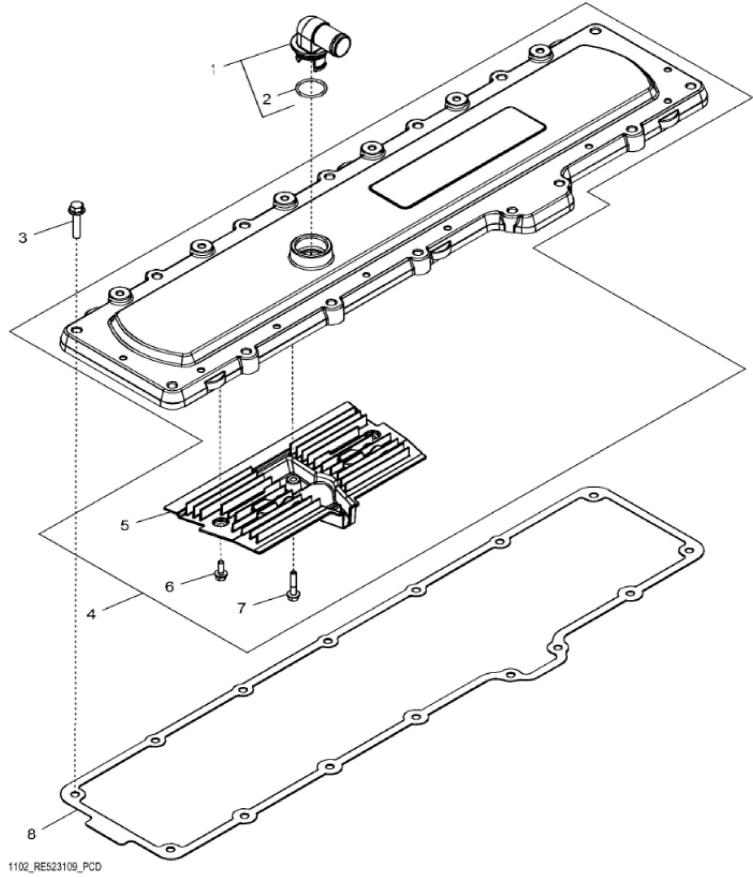
John Deere > Agriculture >TRACTOR >8335R - TRACTOR >8335R Tractor (S.N. 055001-) (Russian Edition) >20 ENGINE 6090RW239-RE564507 >ST130073 - 1102 ROCKER ARM COVER
