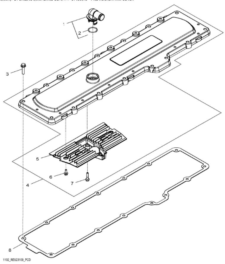
John Deere > Agriculture > TRACTOR > 8270R - TRACTOR > 8270R Tractor (Engine: 6090HBM02, 6090HBM03, Stage II) (South America Edition) > 21 ENGINE 6090HBM02-DZ10414 > ST130073 - 1102 ROCKER ARM COVER
