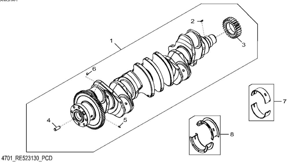
John Deere > Agriculture > TRACTOR > 8345R - TRACTOR > 8345R Tractor (Engine: 6090HBM02, 6090HBM03, Stage II) (South America Edition) > 21 ENGINE 6090HBM02-DZ10414 > ST30568 - 4701 CRANKSHAFT
