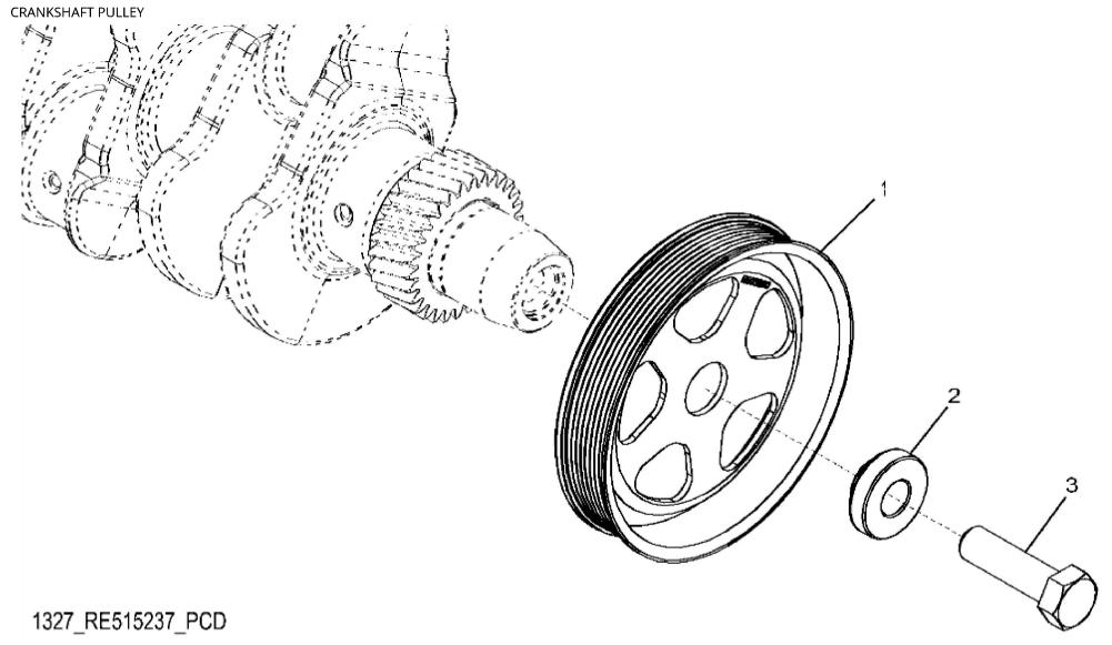
John Deere > Turf And Utility >TRACTOR >4045HLV72 - TRACTOR >5100ML Tractor (Engine 4045HLV72, Final Tier 4)(North American Edition) >20 ENGINE 4045HLV72-RE565006 >ST308624 - 1327 CRANKSHAFT PULLEY
