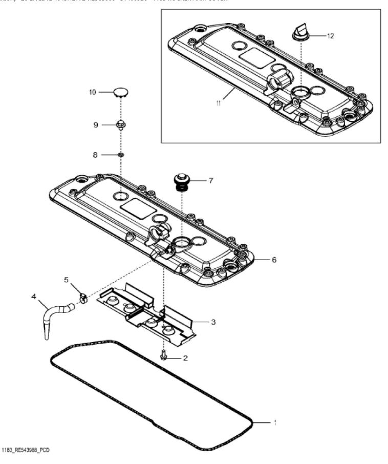
John Deere > Turf And Utility >TRACTOR >4045HLV72 - TRACTOR >5100ML Tractor (Engine 4045HLV72, Final Tier 4)(North American Edition) >20 ENGINE 4045HLV72-RE565006 >ST400926 - 1183 ROCKER ARM COVER
