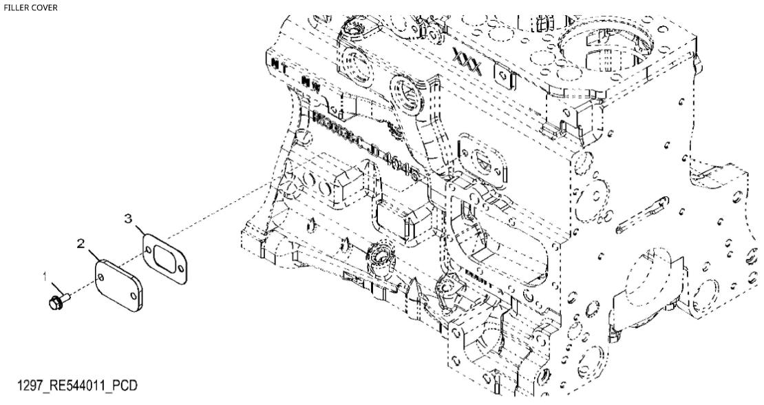
John Deere > Turf And Utility >TRACTOR >4045HLV72 - TRACTOR >5100ML Tractor (Engine 4045HLV72, Final Tier 4)(North American Edition) >20 ENGINE 4045HLV72-RE565006 >ST402282 - 1297 OIL FILLER COVER
