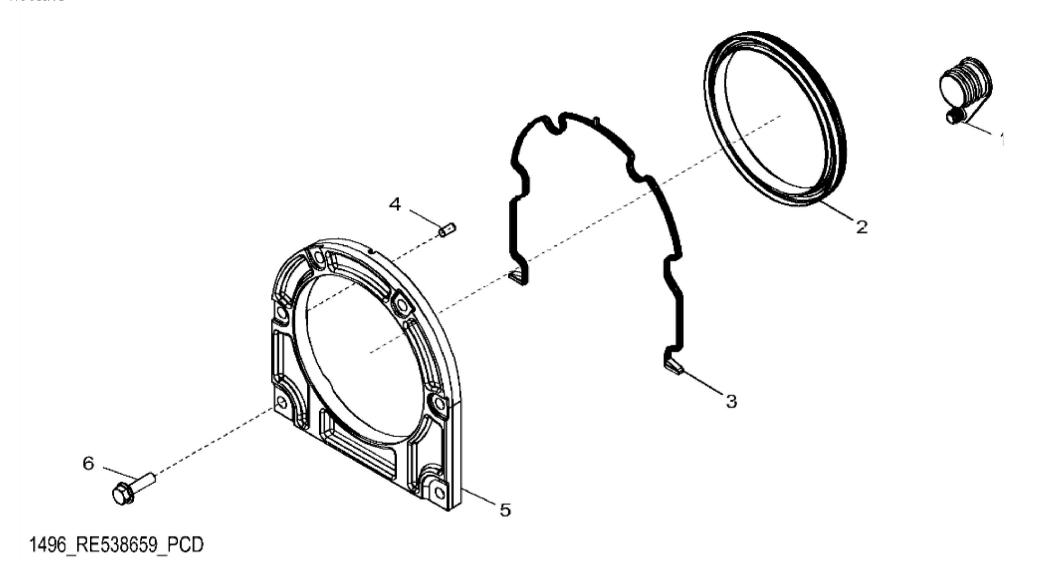
John Deere > Agriculture > TRACTOR > 8400R - TRACTOR > 8400R Tractor (S.N. 115000-)(Worldwide Edition) > 10 ENGINE 6090RW482-DZ102186 > ST122156 - 1496 CRANKSHAFT OIL SEAL AND HOUSING
