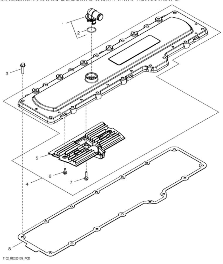
John Deere > Agriculture > TRACTOR > 8270R - TRACTOR > 8270R Tractor (S.N. 100000-)(Engine: 6090HBM02, 6090HBM03, 6090HBM04, 6090HBM05)(South America Edition) > 23 ENGINE 6090HBM02-DZ10414 > ST130073 - 1102 ROCKER ARM COVER
