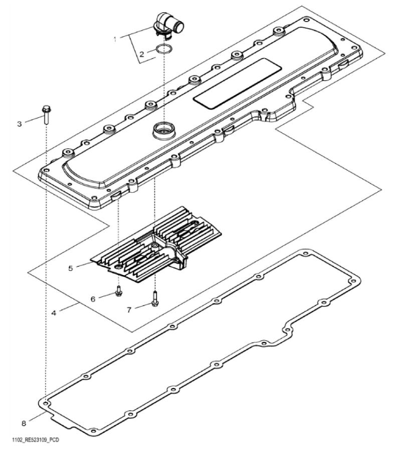
John Deere > Agriculture >TRACTOR >8345R - TRACTOR >8345R Tractor (S.N. 100000-)(Engine: 6090HBM02, 6090HBM03, 6090HBM04, 6090HBM05) (South America Edition) >23 ENGINE 6090HBM02-DZ10414 >ST130073 - 1102 ROCKER ARM COVER
