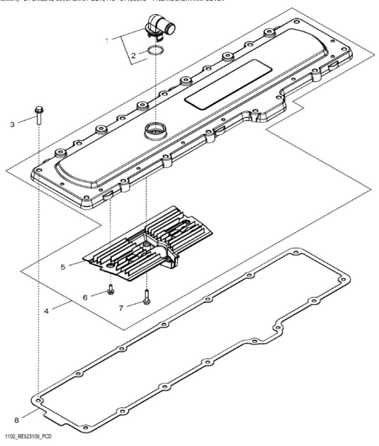
John Deere > Agriculture > TRACTOR > 8370R - TRACTOR > 8370R Tractor (S.N. 100000-)(Engine: 6090HBM01, 6090HBM06) (South America Edition) > 21 ENGINE 6090HBM01-DZ10413 > ST130073 - 1102 ROCKER ARM COVER
