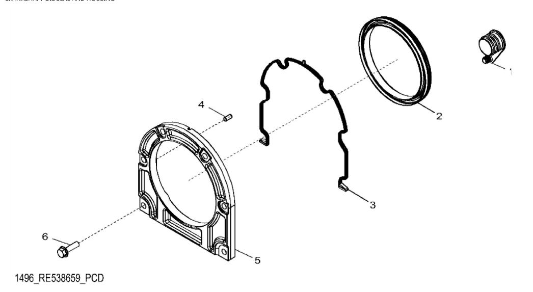
John Deere > Agriculture > TRACTOR > 8370R - TRACTOR > 8370R Tractor (S.N. 100000-)(Engine: 6090HBM01, 6090HBM06) (South America Edition) > 21 ENGINE 6090HBM01-DZ10413 > ST122156 - 1496 CRANKSHAFT OIL SEAL AND HOUSING
