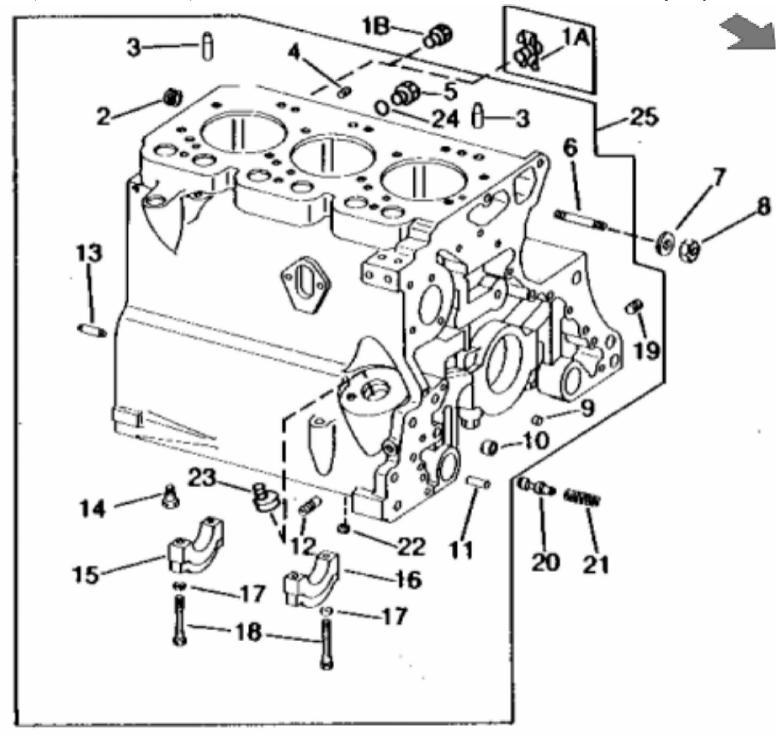
John Deere > Construction And Forestry >BACKHOE, LOADER >300B - BACKHOE, LOADER >300B Loader and Backhoe Loader >10 ENGINE >10-1A - CYLINDER BLOCK [01B03]
