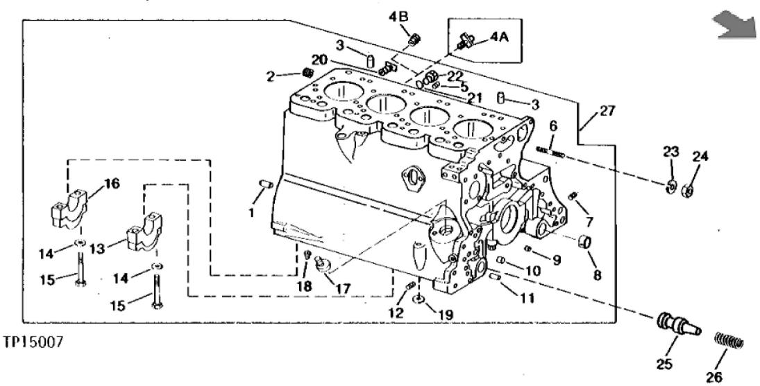
John Deere > Construction And Forestry >BACKHOE, LOADER >401C - BACKHOE, LOADER >401C Loader and Backhoe Loader >10 ENGINE >10-1A - CYLINDER BLOCK [01A22]
