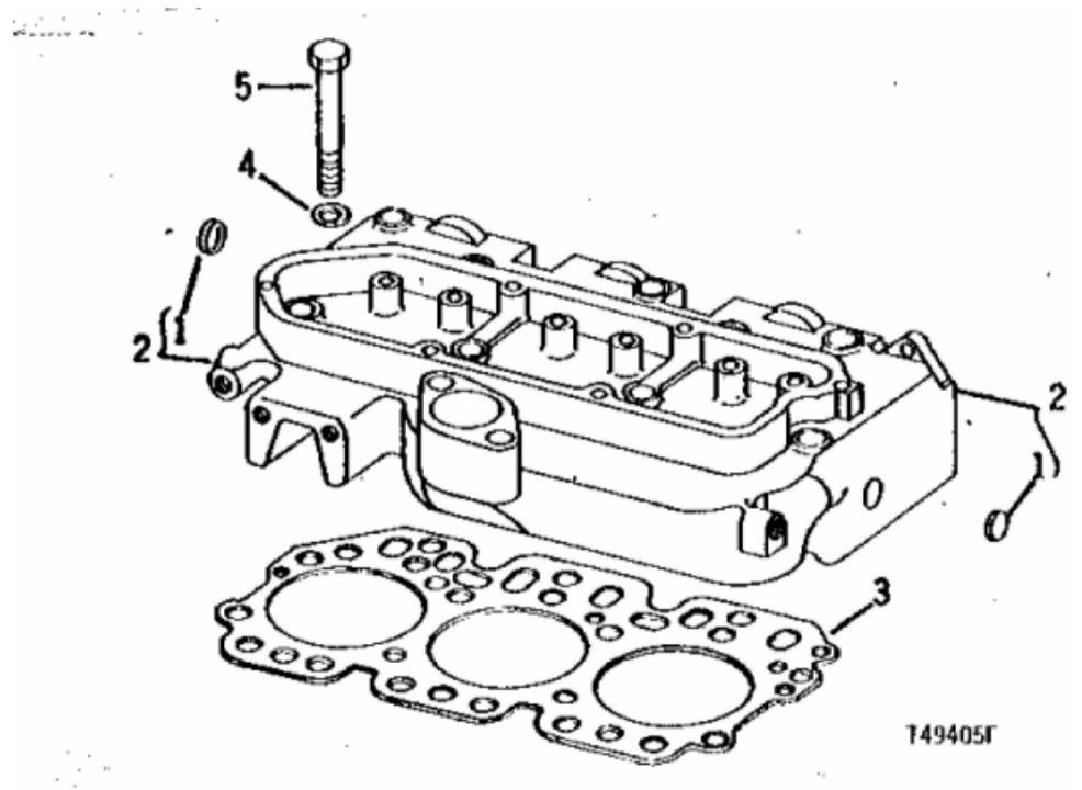
John Deere > Construction And Forestry >BACKHOE, LOADER >302A - BACKHOE, LOADER >302A Loader and Backhoe Loader >10 ENGINE >10-4 - CYLINDER HEAD AND CYLINDER HEAD GASKET [01B07]
