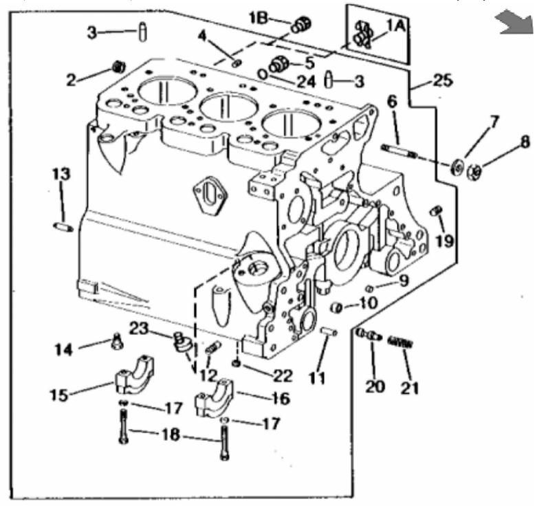
John Deere > Construction And Forestry > BACKHOE, LOADER > 302A - BACKHOE, LOADER > 302A Loader and Backhoe Loader > 10 ENGINE > 10-1A - CYLINDER BLOCK [01B03]
