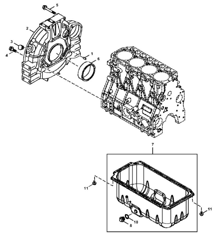
John Deere > Turf And Utility >LOADER, SKID-STEER >324E - LOADER, SKID-STEER >324E Skid Steer Loader (PIN: 1T0324E\_\_\_G297141-) >04 ENGINE, 4TNV98T 4TNV98T-AT408726 >0404 CYLINDER BLOCK 4TNV98T 4TNV98T >ST763899 - FLYWHEEL HOUSING AND OIL SUMP
