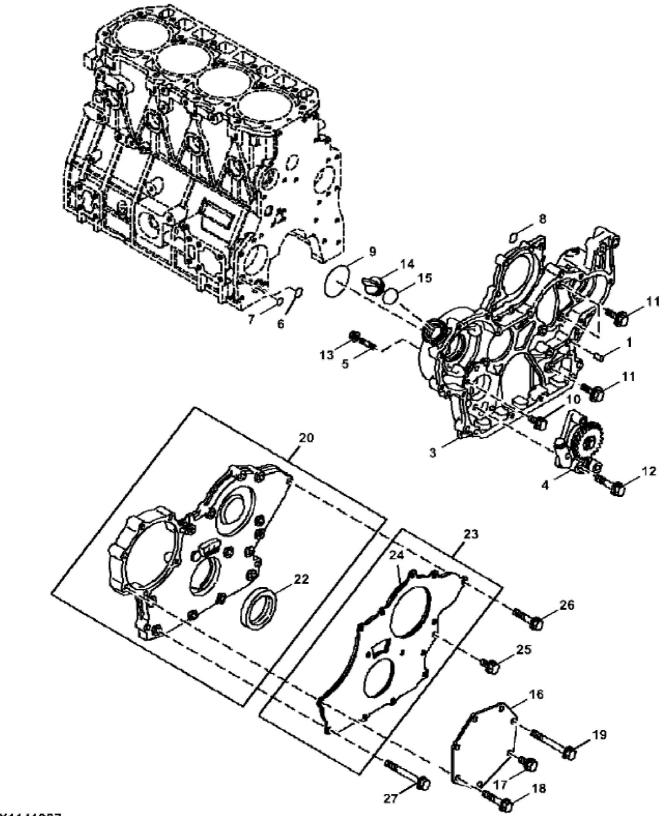
John Deere > Turf And Utility >LOADER, SKID-STEER >324E - LOADER, SKID-STEER >324E Skid Steer Loader (PIN: 1T0324E\_\_\_G297141-) >04 ENGINE, 4TNV98T 4TNV98T-AT408726 >0404 CYLINDER BLOCK 4TNV98T 4TNV98T >ST763939 - GEAR HOUSING
