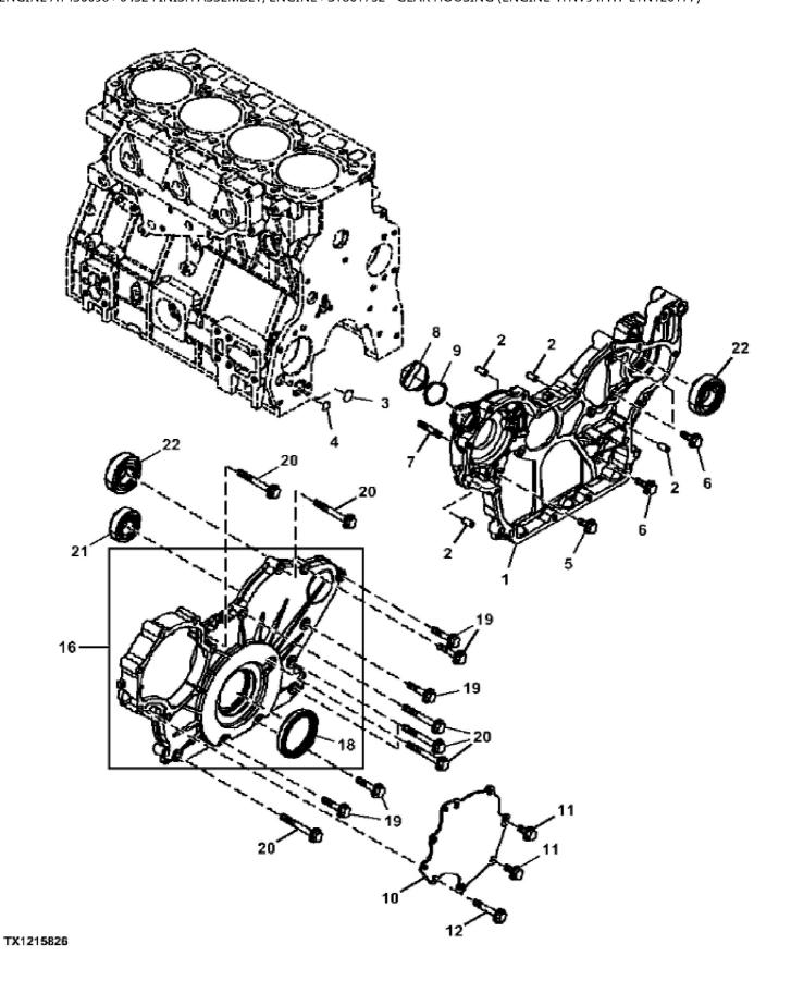
John Deere > Turf And Utility >LOADER, SKID-STEER >332G - LOADER, SKID-STEER >332G Skid Steer Loader (PIN: 1T0332G\_\_\_F300253- ) >04 ENGINE AT436698 >0432 FINISH ASSEMBLY, ENGINE >ST861752 - GEAR HOUSING (ENGINE 4TNV94FHT-ETN120177)
