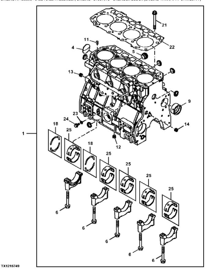
John Deere > Turf And Utility >LOADER, SKID-STEER >332G - LOADER, SKID-STEER >332G Skid Steer Loader (PIN: 1T0332G\_\_\_F300253- ) >04 ENGINE AT436698 >0432 FINISH ASSEMBLY, ENGINE >ST861973 - CYLINDER BLOCK (ENGINE 4TNV94FHT-ETN120177)
