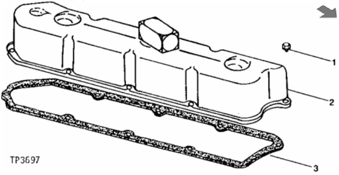
John Deere > Construction And Forestry >BACKHOE, LOADER >410B - BACKHOE, LOADER >410B Backhoe Loader >4 ENGINE 4 >CAMSHAFT AND VALVE ACTUATING MEANS 0402 >0402-5 - ROCKER ARM COVER (WITHOUT TURBOCHARGER) [01E11]
