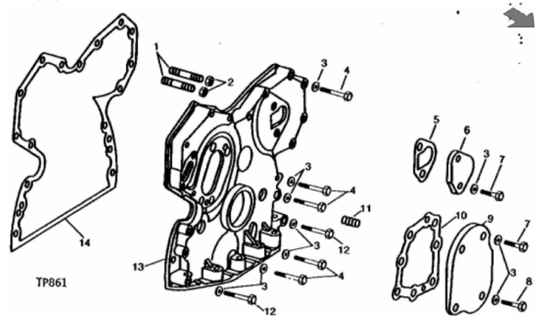
John Deere > Construction And Forestry >BACKHOE, LOADER >410B - BACKHOE, LOADER >410B Backhoe Loader >4 ENGINE 4 >CAMSHAFT AND VALVE ACTUATING MEANS 0402 >0402-6 - TIMING GEAR COVER [01E12]
