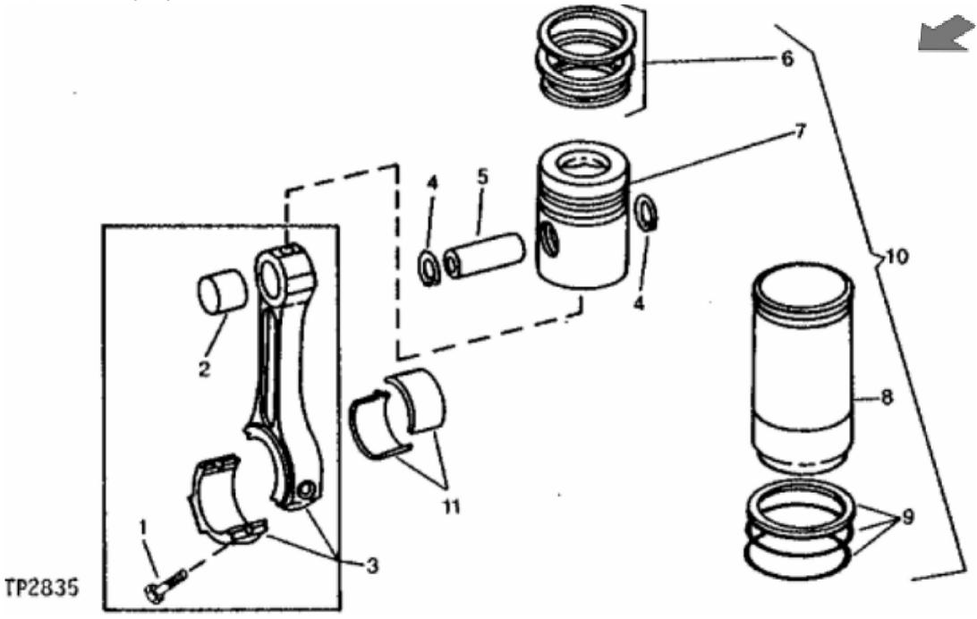
John Deere > Construction And Forestry >BACKHOE, LOADER >410B - BACKHOE, LOADER >410B Backhoe Loader >4 ENGINE 4 >CONNECTING RODS AND PISTONS 0403 >0403-1 - CONNECTING ROD, PISTON, RINGS AND LINER [01E13]
