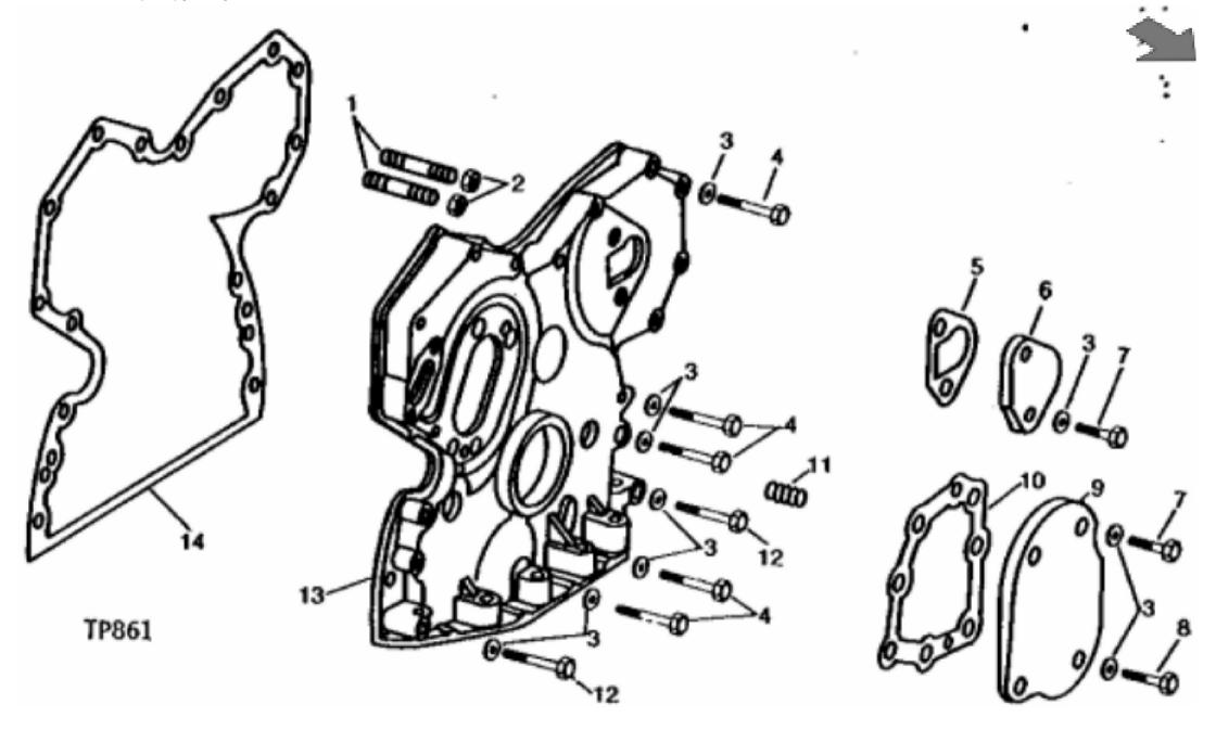
John Deere > Construction And Forestry >BACKHOE, LOADER >710C - BACKHOE, LOADER >710B and 710C Backhoe Loaders >4 ENGINE 4 >CAMSHAFT AND VALVE ACTUATING MEANS 0402 >0402-5 - TIMING GEAR COVER (710B) [02B25]
