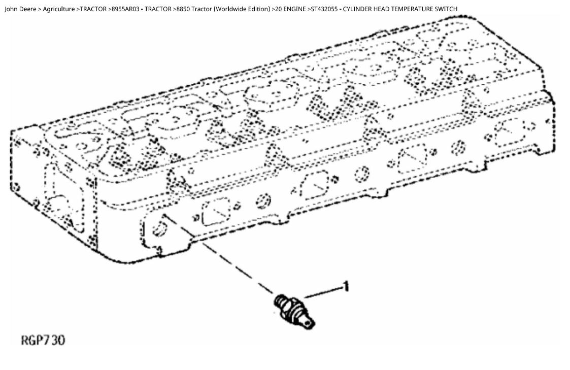
John Deere > Agriculture >TRACTOR >8955AR03 - TRACTOR >8850 Tractor (Worldwide Edition) >20 ENGINE >ST432055 - CYLINDER HEAD TEMPERATURE SWITCH
