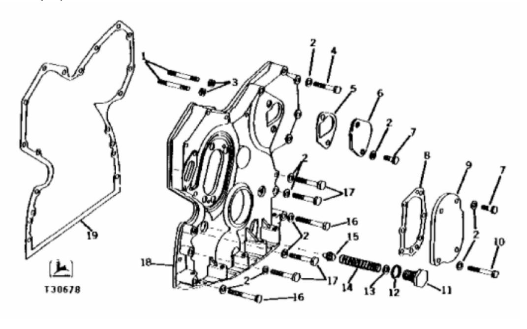
John Deere > Construction And Forestry > BACKHOE, LOADER > 310B - BACKHOE, LOADER > 310A, 310B Backhoe Loaders > 4 ENGINE 4 > CAMSHAFTS AND VALVE ACTUATING MEANS 0402 > 00402-3 - TIMING GEAR COVER [01D03]
