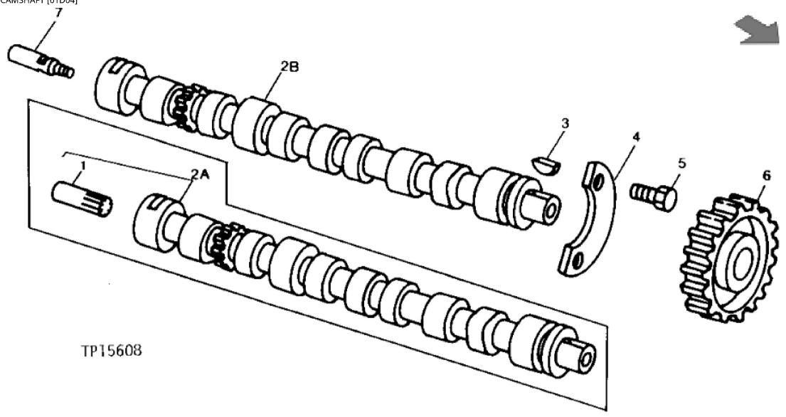
John Deere > Construction And Forestry >BACKHOE, LOADER >310B - BACKHOE, LOADER >310A, 310B Backhoe Loaders >4 ENGINE 4 >CAMSHAFTS AND VALVE ACTUATING MEANS 0402 >00402-4 - CAMSHAFT [01D04]
