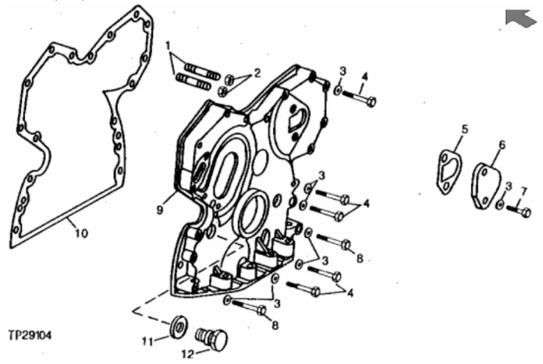
John Deere > Construction And Forestry > BACKHOE, LOADER > 210C - BACKHOE, LOADER > 210C Backhoe Loader > 04 ENGINE 4 > 0402 CAMSHAFT AND VALVE ACTUATING MEANS > ST310687 - TIMING GEAR COVER (300000 - )
