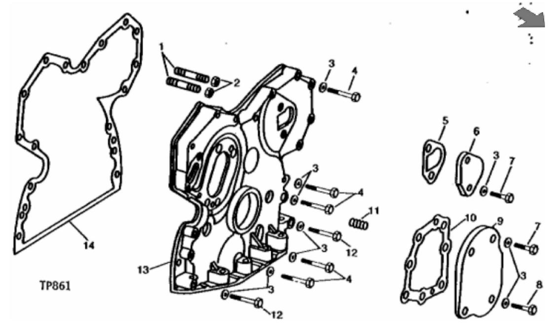
John Deere > Construction And Forestry > BACKHOE, LOADER > 210C - BACKHOE, LOADER > 210C Backhoe Loader > 04 ENGINE 4 > 0402 CAMSHAFT AND VALVE ACTUATING MEANS > ST310686 - TIMING GEAR COVER ( - 299999)
