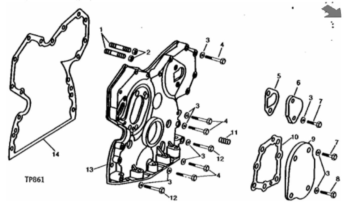
John Deere > Construction And Forestry > BACKHOE, LOADER > 310C - BACKHOE, LOADER > 310C Backhoe Loader > 4 ENGINE 4 > CAMSHAFT AND VALVE ACTUATING MEANS 0402 > 0402-5 - TIMING GEAR COVER (ENGINE SERIAL NO. -299999) [01E20]
