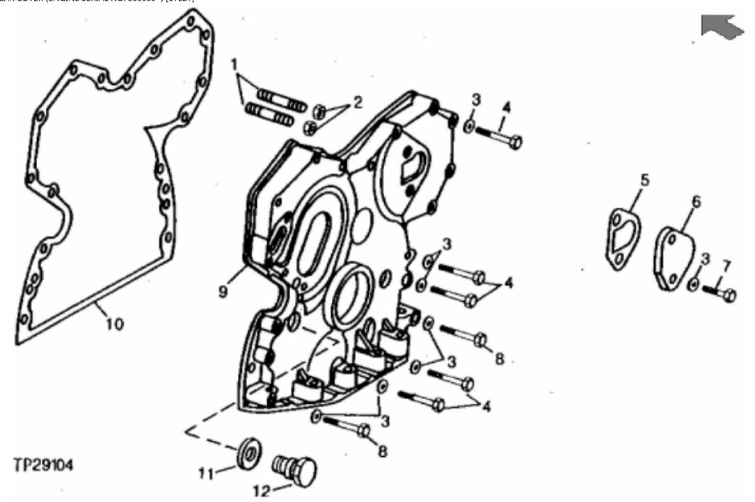
John Deere > Construction And Forestry > BACKHOE, LOADER > 310C - BACKHOE, LOADER > 310C Backhoe Loader > 4 ENGINE 4 > CAMSHAFT AND VALVE ACTUATING MEANS 0402 > 0402-6 - TIMING GEAR COVER (ENGINE SERIAL NO. 300000-) [01E21]
