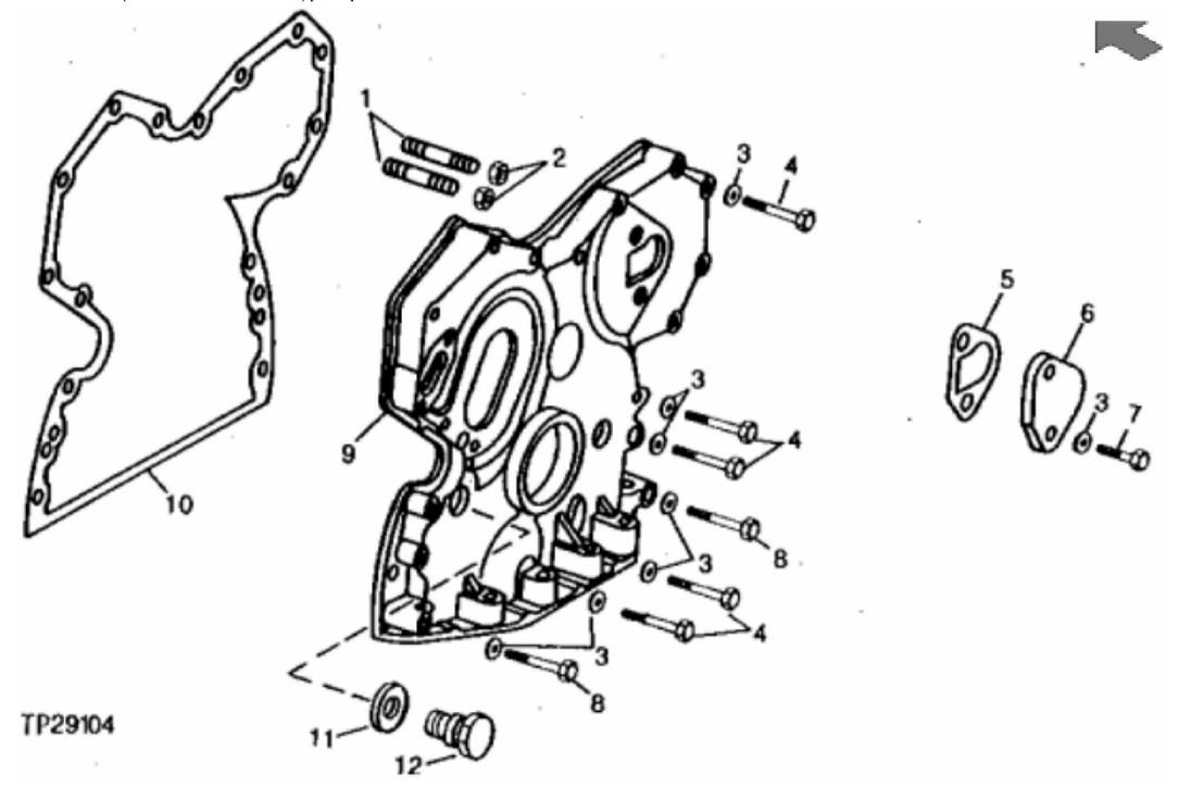
John Deere > Construction And Forestry > BACKHOE, LOADER > 315C - BACKHOE, LOADER > 315C Sideshift Backhoe Loader > 4 ENGINE 4 > CAMSHAFT AND VALVE ACTUATING MEANS 0402 > 0402-6 - TIMING GEAR COVER (ENGINE SERIAL NO. 300000-) [01E21]
