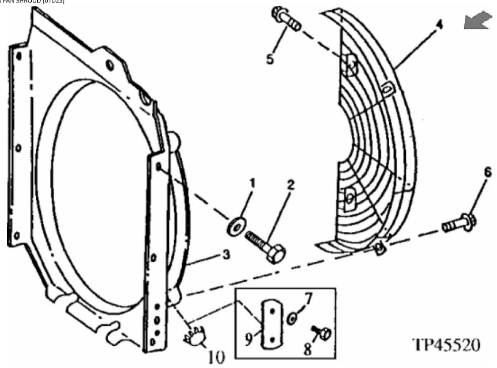
John Deere > Construction And Forestry > BACKHOE, LOADER > 315CH - BACKHOE, LOADER > 315CH Sideshift Backhoe Loader > 5 ENGINE AUXILIARY SYSTEM 5 > COOLING SYSTEMS 0510 > 0510-3 - RADIATOR FAN SHROUD [01D23]
