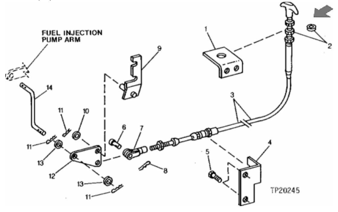
John Deere > Construction And Forestry > BACKHOE, LOADER > 315CH - BACKHOE, LOADER > 315CH Sideshift Backhoe Loader > 5 ENGINE AUXILIARY SYSTEM 5 > SPEED CONTROLS 0515 > 0515-4 - ENGINE STOP CABLE [01E01]
