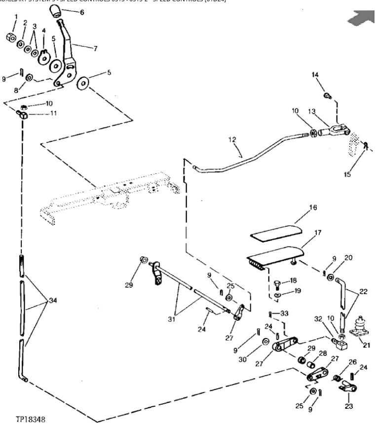
John Deere > Construction And Forestry > BACKHOE, LOADER > 315CH - BACKHOE, LOADER > 315CH Sideshift Backhoe Loader > 5 ENGINE AUXILIARY SYSTEM 5 > SPEED CONTROLS 0515 > 0515-2 - SPEED CONTROLS [01D24]
