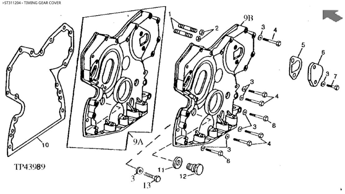
John Deere > Construction And Forestry >BACKHOE, LOADER >315D - BACKHOE, LOADER >300D, 310D and 315D Backhoe Loader >04 ENGINE >0402 CAMSHAFT AND VALVE ACTUATING MEANS >ST311204 - TIMING GEAR COVER
