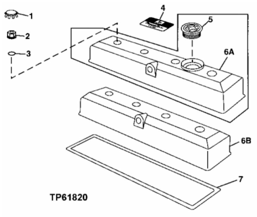
John Deere > Construction And Forestry > BACKHOE, LOADER > 410E - BACKHOE, LOADER > 410E Backhoe Loader > 04 ENGINE > 0402 CAMSHAFT AND VALVE ACTUATING MEANS > ST273325 - ROCKER ARM COVER
