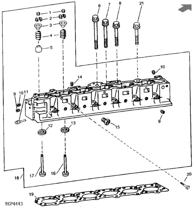
John Deere > Agriculture >TRACTOR >8410T - TRACTOR >8110T, 8210T, 8310T and 8410T Tractors (Worldwide Edition) >20 ENGINE >ST422963 - CYLINDER HEAD
