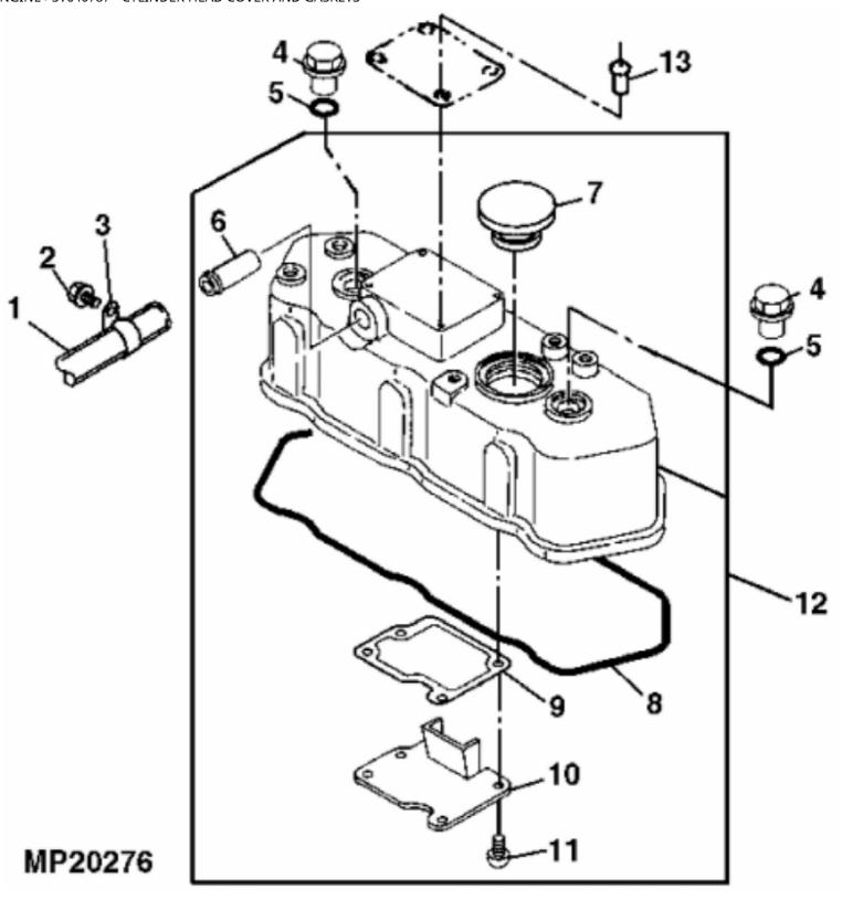
John Deere > Turf And Utility >TRACTOR, COMPACT UTILITY >4110 - TRACTOR, COMPACT UTILITY >4110 Compact Utility Tractor >20 ENGINE >ST640787 - CYLINDER HEAD COVER AND GASKETS
