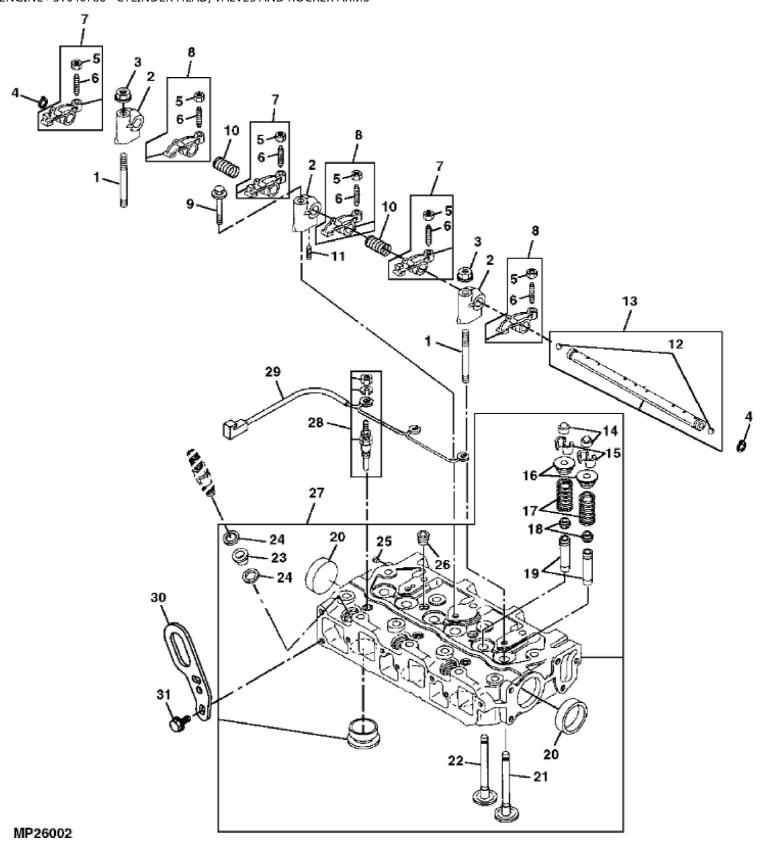
John Deere > Turf And Utility >TRACTOR, COMPACT UTILITY >4110 - TRACTOR, COMPACT UTILITY >4110 Compact Utility Tractor >20 ENGINE >ST640786 - CYLINDER HEAD, VALVES AND ROCKER ARMS
