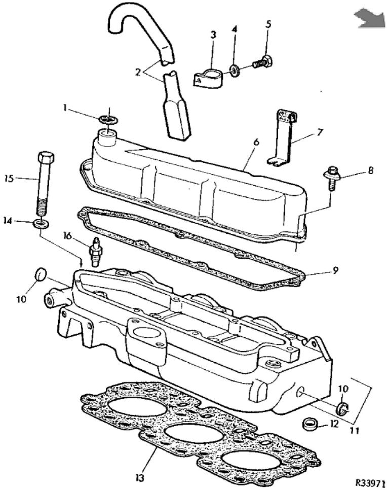
John Deere > Turf And Utility > TRACTOR > 2240 - TRACTOR > 2240 ( -349999) Tractor > 20 ENGINE > 20-4 - CYLINDER HEAD AND ROCKER ARM COVER [01A20]
