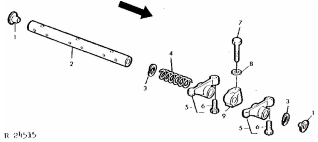
John Deere > Turf And Utility >TRACTOR >2240 - TRACTOR >2240 ( -349999) Tractor >20 ENGINE >20-6 - ROCKER ARM SHAFT [01A22]
