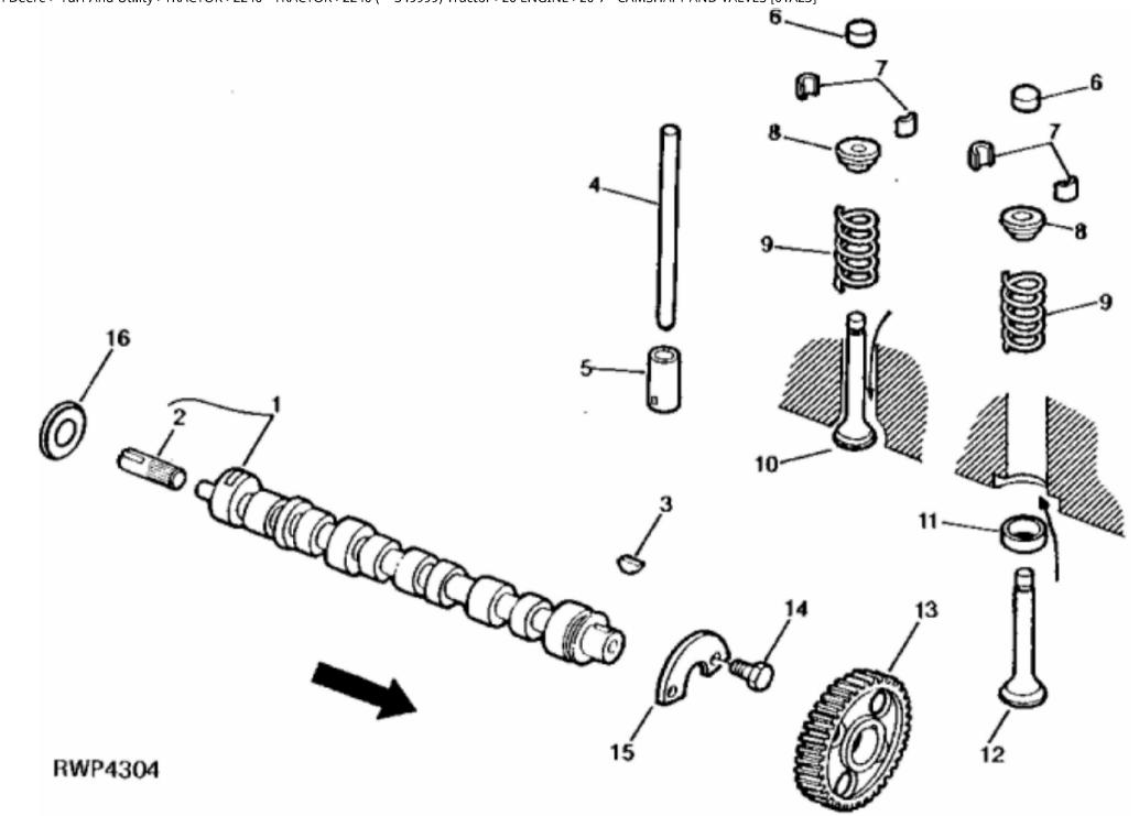
John Deere > Turf And Utility >TRACTOR >2240 - TRACTOR >2240 ( -349999) Tractor >20 ENGINE >20-7 - CAMSHAFT AND VALVES [01A23]
