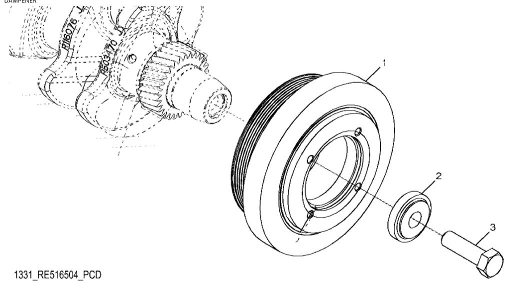
John Deere > Agriculture > TRACTOR > SE6920 - TRACTOR > SE6920 Tractor (Europe Edition) > 20 ENGINE 6068TL074-DD21494 - DD21761 > ST633630 - 1331 CRANKSHAFT PULLEY AND TORSIONAL DAMPENER
