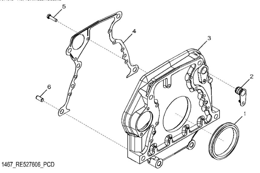
John Deere > Turf And Utility >TRACTOR >3029HPY50 - TRACTOR >5075E Tractor (Tier3)(9X3 TSS Transmission and Collar Shift Transmission W/ OOS)(India Edition) >20 ENGINE RE-RE547278 >ST614045 - 1467 FLYWHEEL HOUSING
