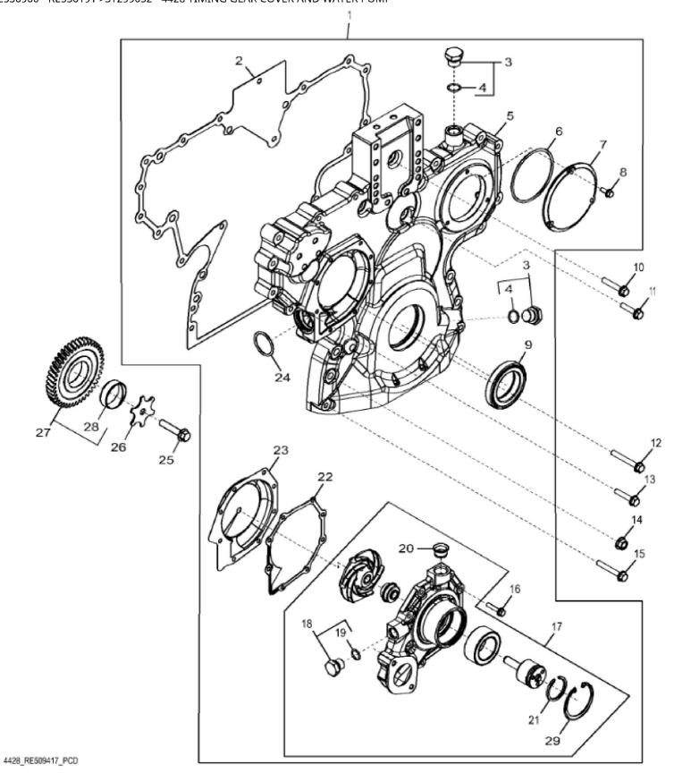
John Deere > Turf And Utility >TRACTOR >4045TP079 - TRACTOR >5076EF (Narrow) Tractor (Worldwide Edition) >20 ENGINE 4045DP057-RE530900 - RE556191 >ST299032 - 4428 TIMING GEAR COVER AND WATER PUMP
