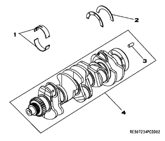
John Deere > Turf And Utility >LOADER, SKID-STEER >5030HT001 - LOADER, SKID-STEER >332 Skid Steer >20 ENGINE 5030HT001-RE509090 >ST150337 - 4702 (CRANKSHAFT / BEARINGS)
