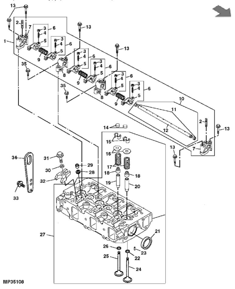
John Deere > Turf And Utility >TRACTOR, COMPACT UTILITY >3TNV84HT - TRACTOR, COMPACT UTILITY >3720 Compact Utility Tractor >20 ENGINE (MARKED 3TNV84HT-JT, -JTE) >ST349140 - CYLINDER HEAD, VALVES AND ROCKER ARMS
