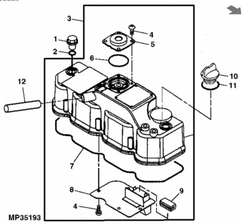
John Deere > Turf And Utility >TRACTOR, COMPACT UTILITY >3TNV84HT - TRACTOR, COMPACT UTILITY >3720 Compact Utility Tractor >20 ENGINE (MARKED 3TNV84HT-JT, -JTE) >ST349141 - CYLINDER HEAD COVER AND GASKETS
