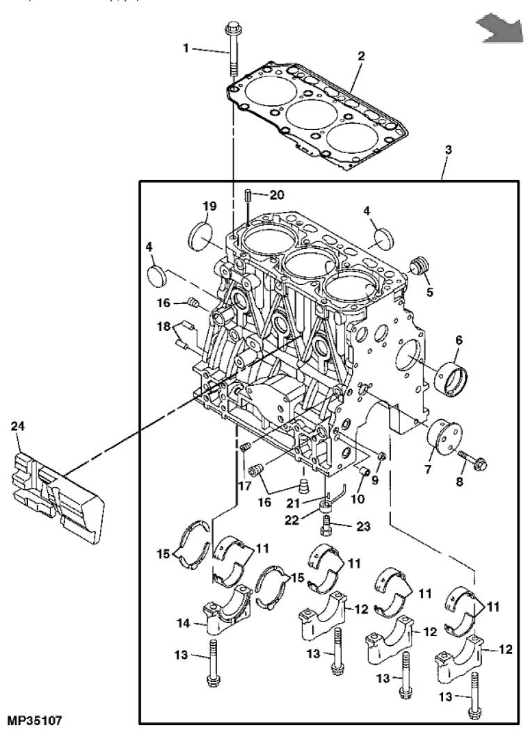
John Deere > Turf And Utility >TRACTOR, COMPACT UTILITY >3TNV84HT - TRACTOR, COMPACT UTILITY >3720 Compact Utility Tractor >20 ENGINE (MARKED 3TNV84HT-JT, -JTE) >ST349139 - CYLINDER BLOCK AND MAIN BEARINGS
