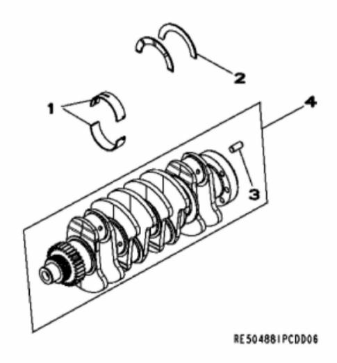
John Deere > Turf And Utility >TRACTOR, COMPACT UTILITY >4320 - TRACTOR, COMPACT UTILITY >4320 Compact Utility Tractor >20 ENGINE 4024TLV01-RE516053 >ST293065 - 4701 CRANKSHAFT / BEARINGS
