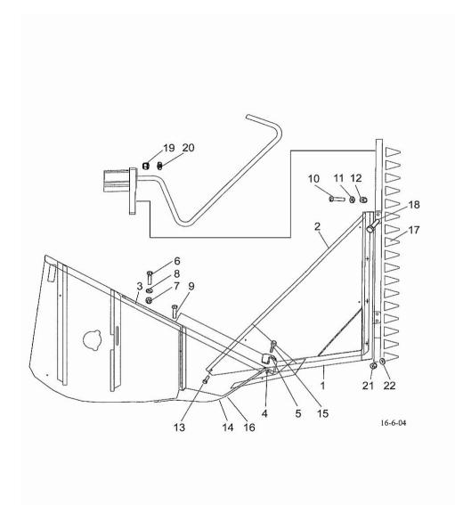
Section: Cutting table and feeding elevator VERTICAL BLADES, DX/RH/RE
