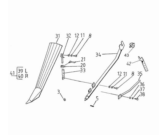
Section: Cutting table and feeding elevator SHORT DIVIDERS, WB
