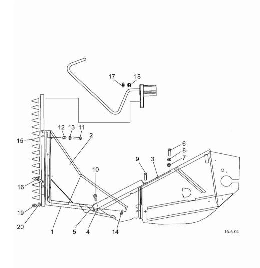
Section: Cutting table and feeding elevator VERTICAL BLADES, SX/LH/LI
