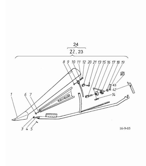
Section: Cutting table and feeding elevator LONG DIVIDERS, WB
