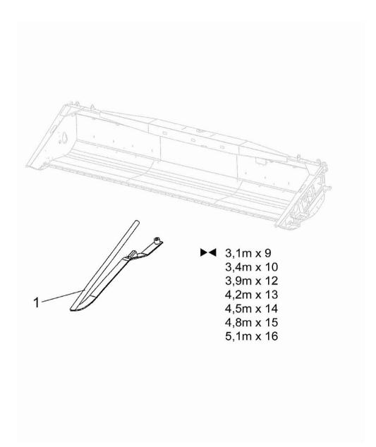
Section: Cutting table and feeding elevator **EARLIFTERS**
