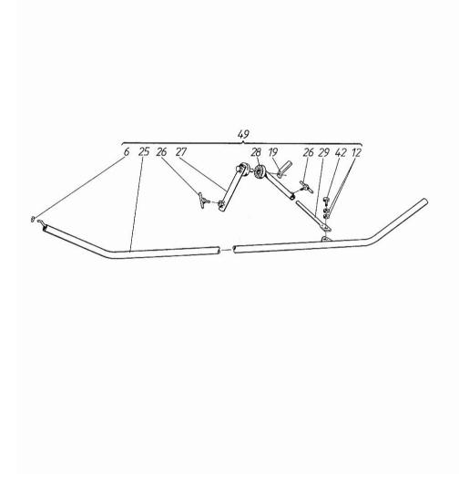
Section: Cutting table and feeding elevator **SIDETUBE**
