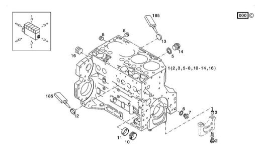
Section: B0 - ENGINE CRANKCASE
