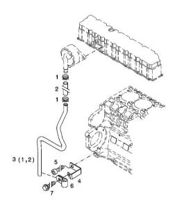
Section: B0 - ENGINE **BLEEDING TUBE**
