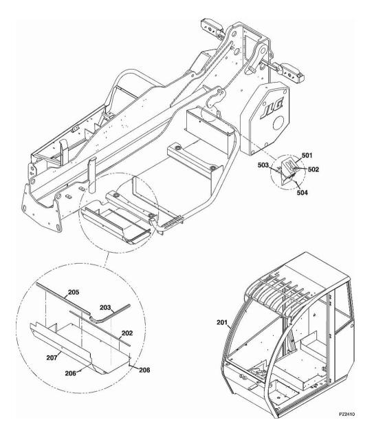
Section: FRAME & ATTACHING PARTS
