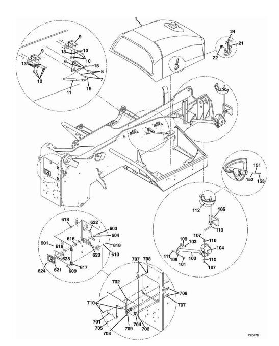
Section: FRAME & ATTACHING PARTS
