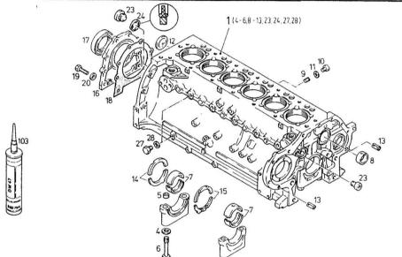
Section: ENGINE CRANK CASE
