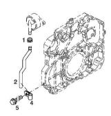
Section: B0 - ENGINE **BLEEDING TUBE**
