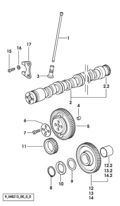
Section: ENGINE CAMSHAFT
